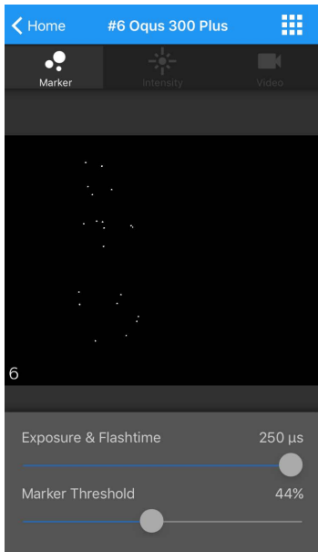
Figure 2: Screenshot from the ViewFinder app showing the detail view with settings for a single camera in the motion capture system.
