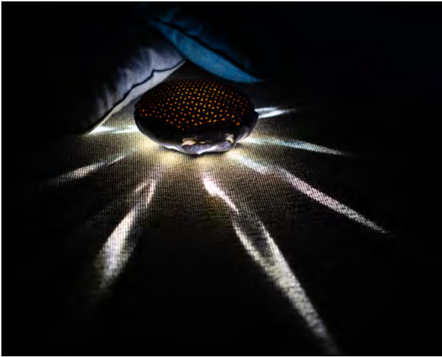
Figure 3: Light scattered through laser-cut slits underneath, radiating in the environment, amplifies the user’s sense of their own subtle movements as they hold Azalea.
